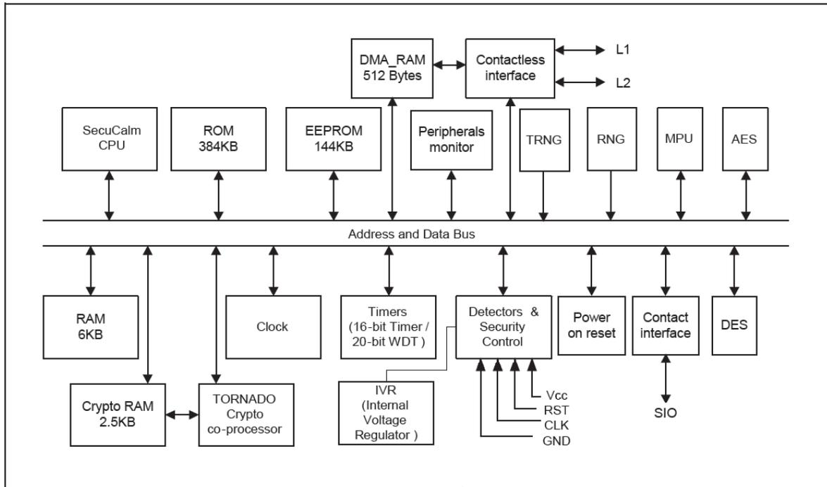
**Figure 3 IC Chip Hardware Composition Diagram**
