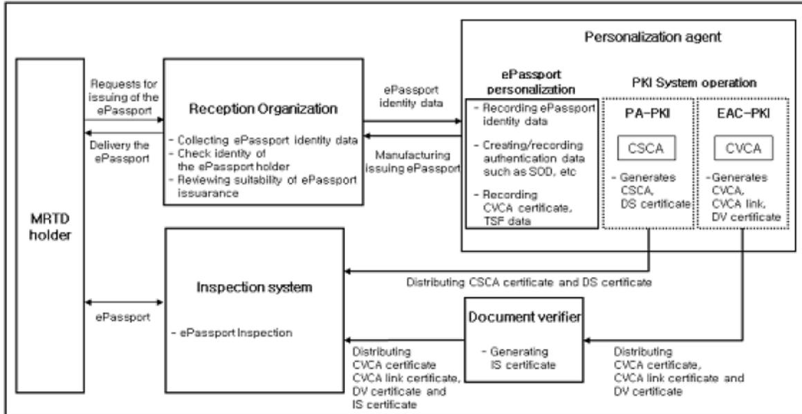
**Figure 2 Entire Composition Diagram of ePassport System**
